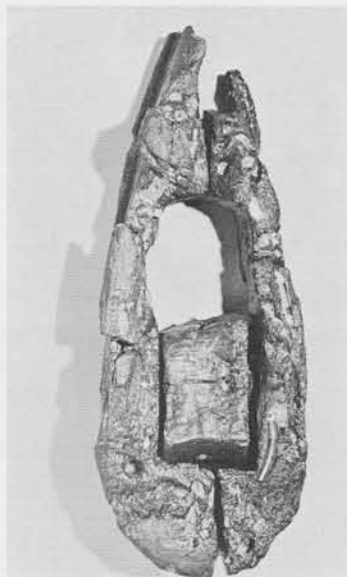
Wooden pulley, badly attacked by teredo worms, had fallen beside the mast step. Probably the sailors used it to raise and lower the ship's yard.
