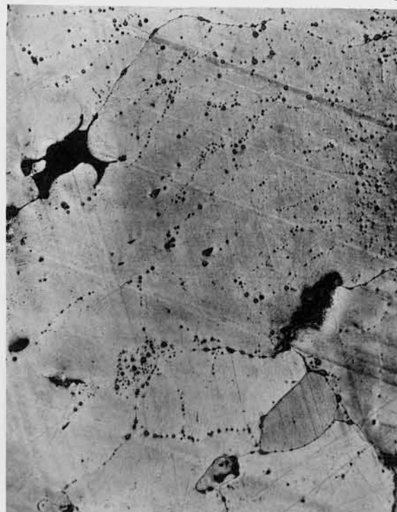
2 Micrograph taken with the scanning electron microscope (300 X) of a piece from fragment of oxhide ingot found at Ayia Irini, on the Island of Keos. The date is Late Minoan IB or 1500-1450 B.C. The even grain structure of this very pure copper shows clearly in this sample cut off with a hacksaw.
