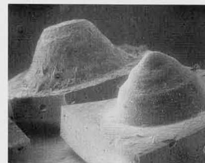
8a The leading edge of a drill hole shows a most revealing shape and clue to the type of drill used. This may vary from flat to somewhat rounded and occasionally angular. The scanning micrograph was made from drill holes on the engraved surface of a Group 1 seal.
