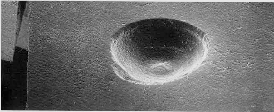
14b Results of experimental drilling on hematite using a copper ball drill and a water slurry of emery.
