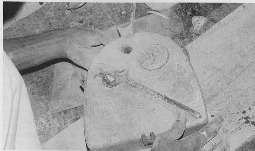
14 When the first half of the mold impression has been produced, ashes are sprinkled over the top of the sand, in the impression, and over the wax image. The other half of the mold will be placed over this one and packed with sand to produce an impression in it also (here the two wax images are a trident and a small disk).
