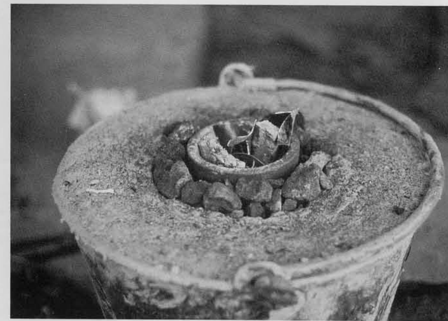
10 The crucible is packed into coals and filled with scrap metal ready for melting.
