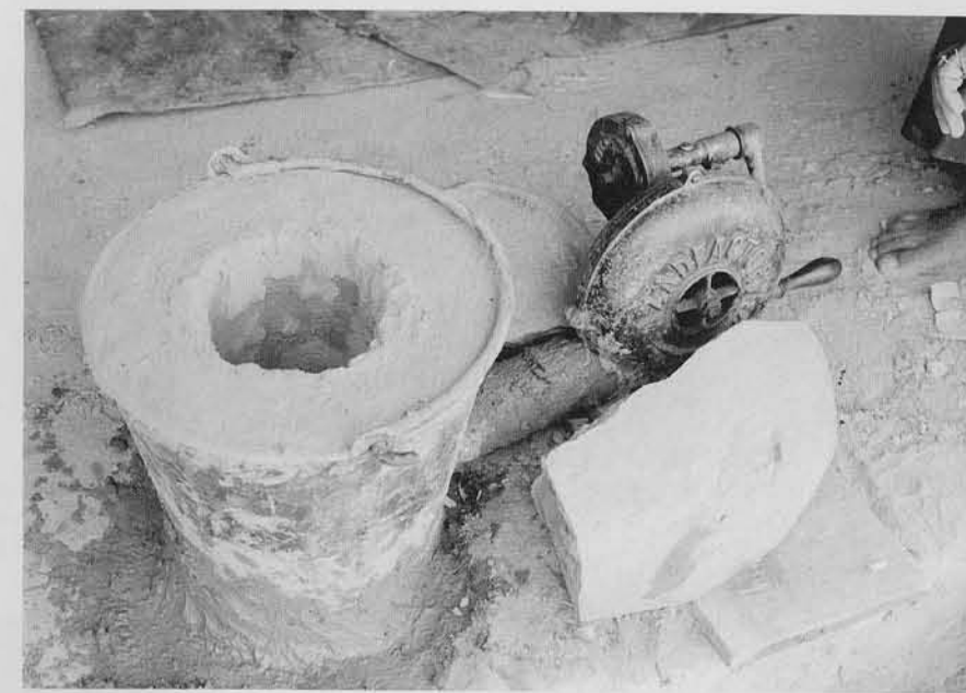
9 Completed furnace assembly with handpowered air pump supported by large rocks on each side.
