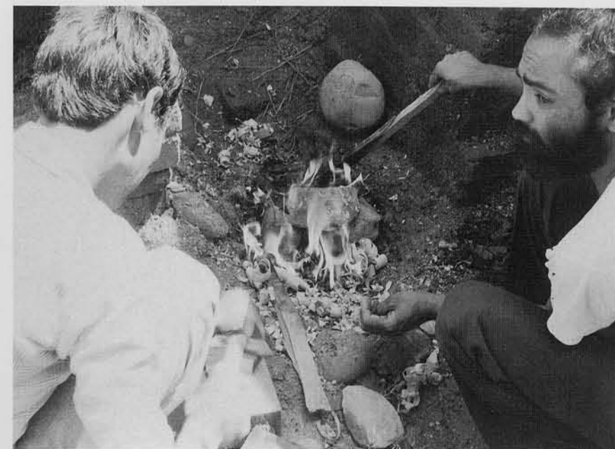
6 The wax model inside the investment is melted out by immersing the mold in a fire at the casting site.
