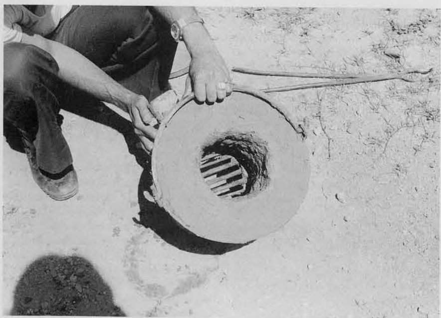
8 Appearance of the inside of the bucket furnace showing the small opening into which fuel and the crucible are placed.
