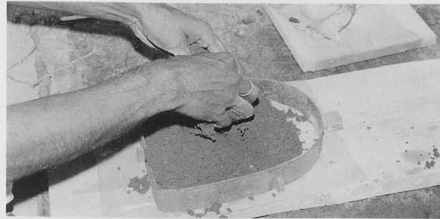
13 The sand mixture is packed into the bottom half of the mold first, around the wax image that is to be reproduced in metal. The object in the right background is a block of wood that will later be used as a stand on which to place the mold.
