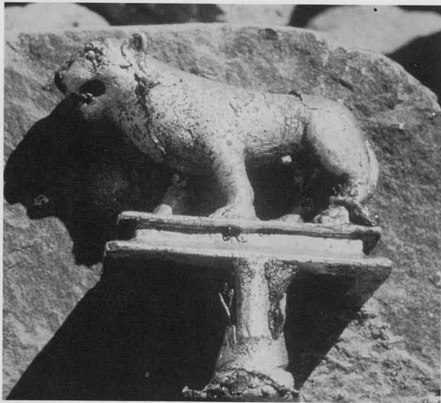
11 A newly cast object showing the presence of a casting skin and surface irregularities that will need to be smoothed by filing. The protrusion on the bottom of the piece was formed by metal which cooled in the runner and riser channels, and will be cut off and filed down so that the statue will stand flat on its base.
