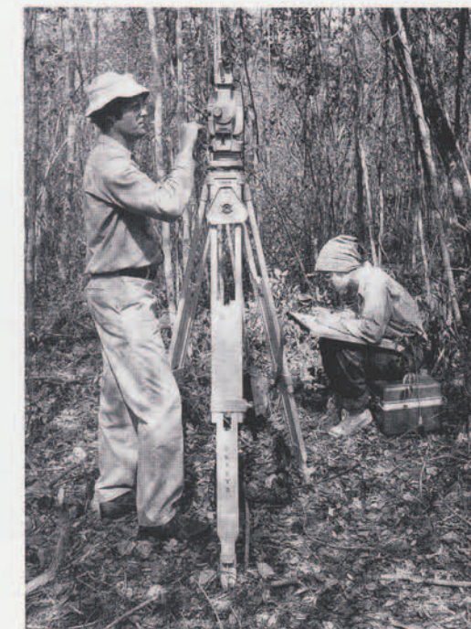
FIG. 4. Drs. Gair Tourtellot and Patricia McAnany using an EDM Total Station during settlement mapping at Sayil. New technologies such as this contribute to the increasingly sophisticated survey methods that mark recent field research in the Maya lowlands.
