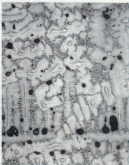
This is a bronze with tin levels of 10%–18% that was cast and received no further work. The long arm-like dendrites are clearly seen.
