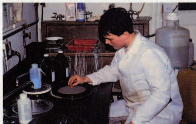
A student is polishing a mounted and ground sample on a polishing wheel.
