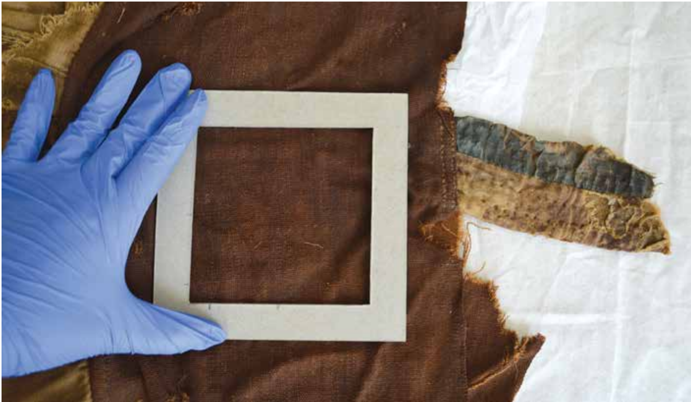
Thread count is an important metric in textile analysis. Here, I use a cardboard viewfinder to count the threads in a wool garment with a silk strap.
